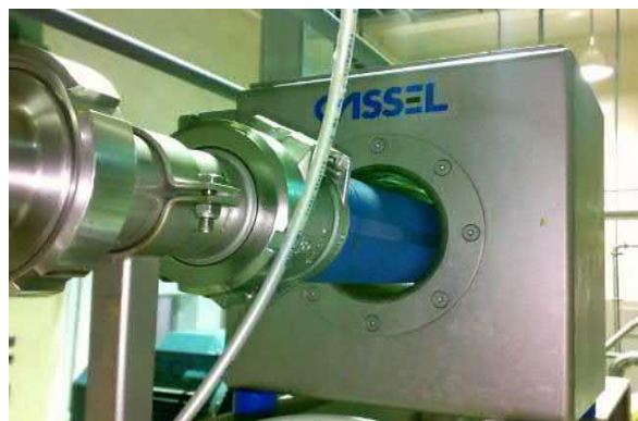
The pressure hose guarantees stability even at pressures up to 16 bar. For higher pressure up to 40 bar, pipe sections made of POM are used.
